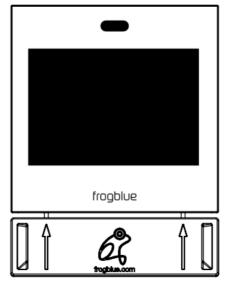
Put the unlocking tool on the bottom of the Display. Please notice that the pins of the unlocking tool are fully inserted in the 2 holes on the bottom of the display. The frogblue logo must
