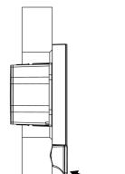
Push the unlocking tool on the bottom side towards the wall and slightly upwards.
