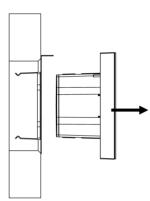
Touch the display laterally and remove it out of the holder.
